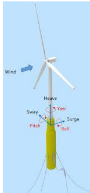
Figure 5: Degrees of freedom of Floating Wind Turbine Installation
