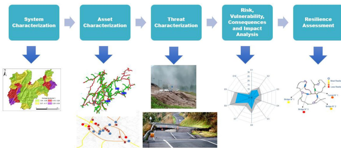
Fig. 8 The five-step approach for a resilience assessment is presented here schematically. The spatial factor is crucial from the beginning, as the system and asset characterization are referring to regional (ter-
